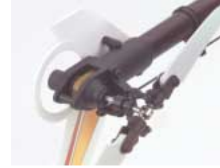
The Venture's ball bearing-supported belt drive is hard to top when it comes to ease of tail rotor setup and reduction of maintenance.
