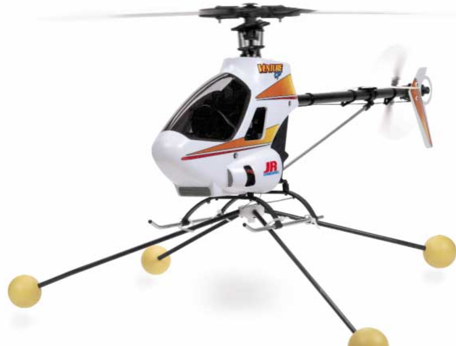
The efficiency and mechanical simplicity afforded by the Venture's CCPM electronic mixing pays off in extended control precision and greatly reduced wear.
